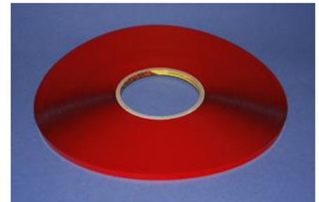
Full adhesive strength of the tape sets in after roughly 72 hours, given a surface temperature of 20°C.
